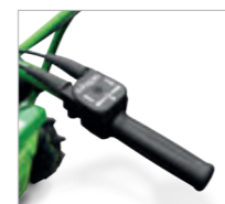
Rotary handle for direction and speed adjustment
