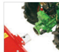
Pipe mounting flange: easy and fast changing of attachments
