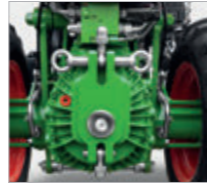
Attachment coupling by Agria: easy and fast changing of attachments
