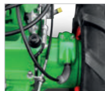
Robust steering brake clutch for easy steering
