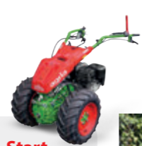
Portal-axle to adjust centre of gravity
