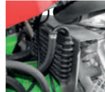
Additional oil cooler for use even at high temperatures
