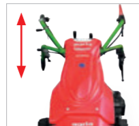
Height adjustment of handle bar without tools
