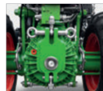
Attachment coupling by Agria: Change attachments easy and fast
