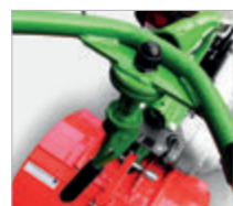
Quick-adjustment lever for shifting side of handle bar
