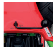
Safe storing of the machine with central locking brake
