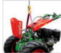
Safe loading with lifting sling and eye bolts
