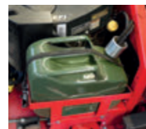
Removable-fuel- tank-system by Agria, fuel level display on remote
