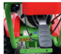
Drive forward / backward, easily switchable via foot pedal
