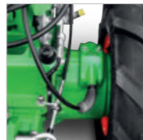
Robust steering brake clutch for easy steering
