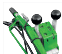
Shift gears and driving direction directly on the handle bar
