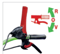
Safe gear change by one-hand operation
