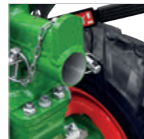
Additional fixture for towed attachments, e.g. ploughs
