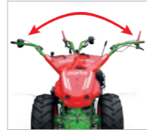
Handlebar can be easily adjusted laterally
