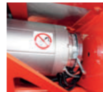
Electromechanical brake for safety on slopes
