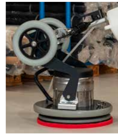
Tilting drawbar for increasing the contact pressure.
