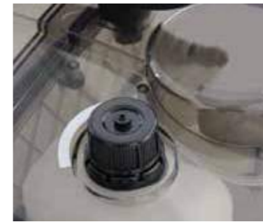
A separate tank allows for the use of anti-foaming agent and guarantees problem-free work.
