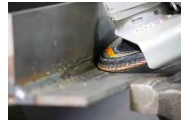
Can be individually adapted by grinding down the flap backing.
